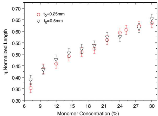
Fig. 1. The shrinking of a NIPA gel sheet as a function of its monomer concentration. The normalized length was obtained by dividing the diameter of a warm gel disc by its original diameter. Shrinking was obtained by immersing the discs into a water bath and increasing the temperature up to 45 °C over ten hours.  $t_0$  is the thickness of the cold sheet.
